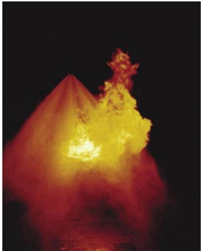
Local application fire test with HI-FOG high pressure water mist.
